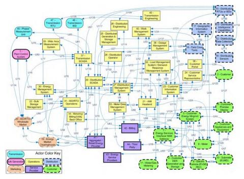
Exhibit 4.4.2 Architectures Such as the Smart Grid Example Shown Here, are Increasingly Complex and Interconnected across Multiple Domains
