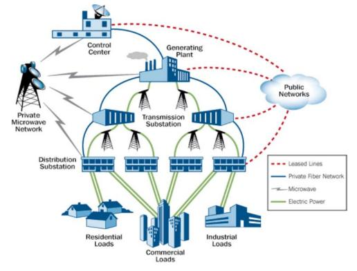
Exhibit D.1 Overview of the Electric Power System and Control Communications
